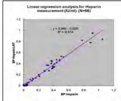
**Conclusion**: Well correlated results between both devices on STAR, for UFH or LMWH measurement. Untreated samples measured as expected <0.05 IU/ml.
