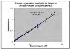
**Conclusion:** excellent correlation of the results obtained with both devices for heparin measurement. Inter assay CV% verification is also satisfying.
