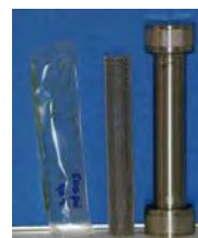
Fig. 2: Rapid Dialysis Procedure (RDP); the picture on the left side shows the polyethylene membrane bag, the steel mesh and the ASE-cell; right side: principle of RDP during the dialysis process
